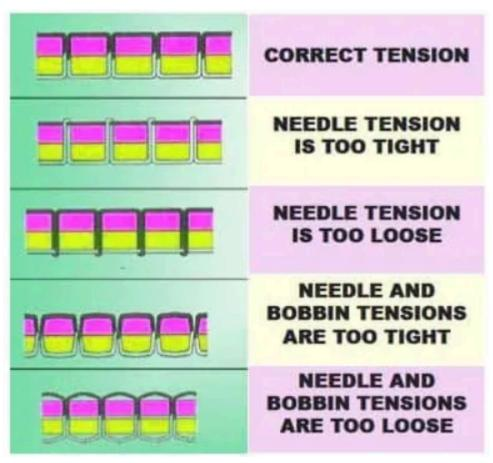
The bottom two examples will be rare and will need a service engineer to resolve as the bobbin tension will need assessing.
